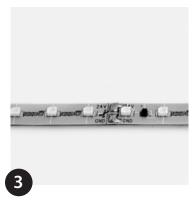
Press in position, avoiding direct pressure on LEDs.
